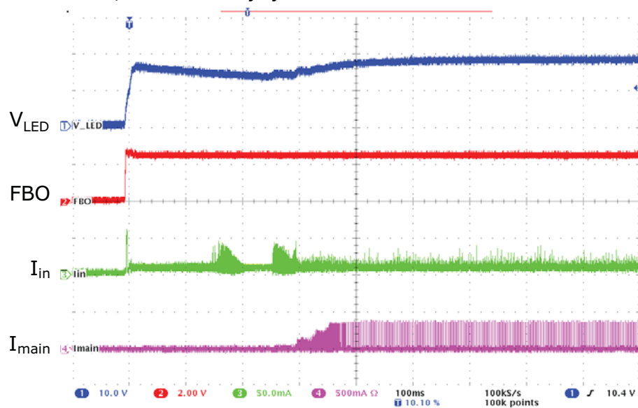
Figure 5-1. START-UP behavior, PWM = 10% duty cycle.
