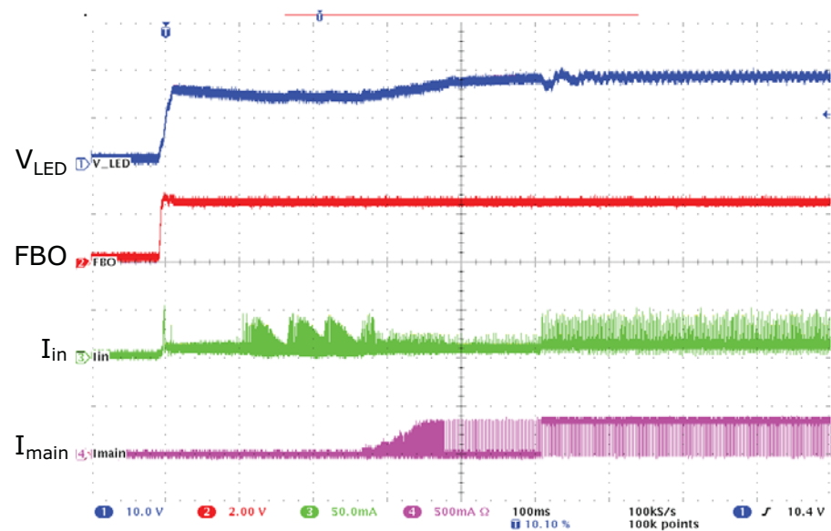
Figure 5-2. START-UP behavior, PWM = 90% duty cycle.
