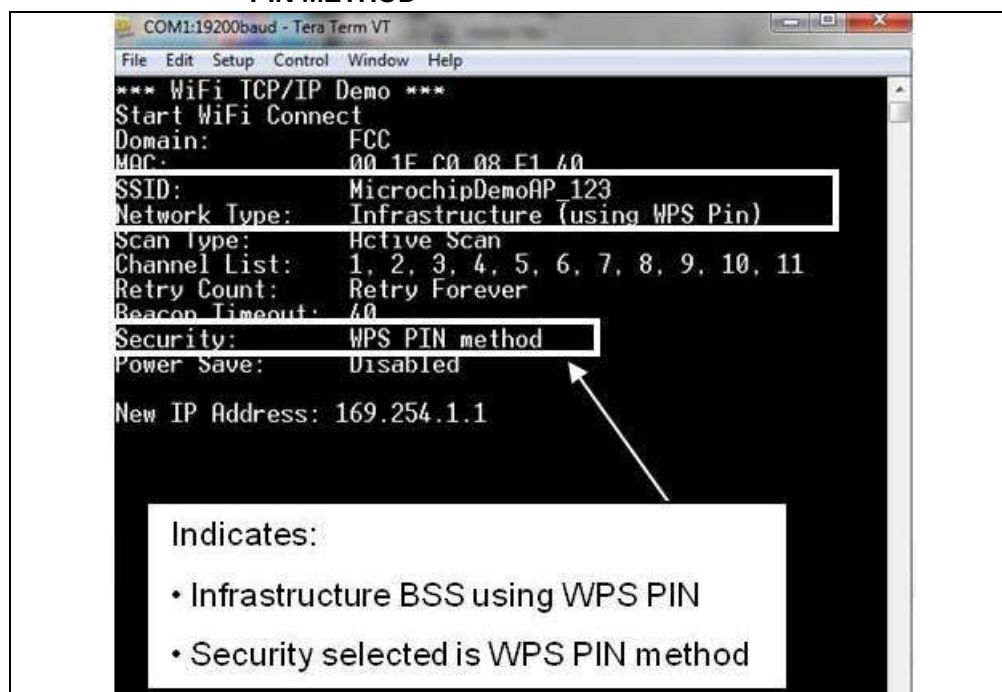
FIGURE 4-49: DEVELOPMENT BOARD SERIAL OUTPUT DISPLAY: WPS PIN METHOD
