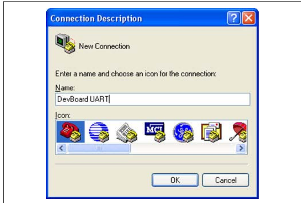
FIGURE 2-9: HYPERTERMINAL NAME SETUP
