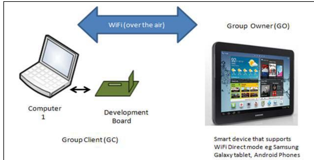
FIGURE 4-36: WIFI DIRECT ENVIRONMENT SETUP
