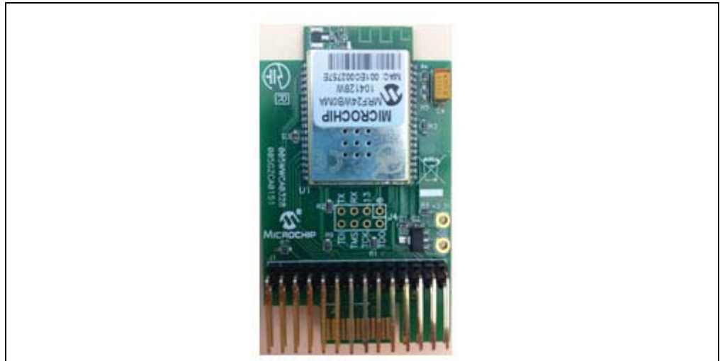
FIGURE 2-1: MRF24WB0MA/B OR MRF24WG0MA/B WI-FI® PICTAIL™
