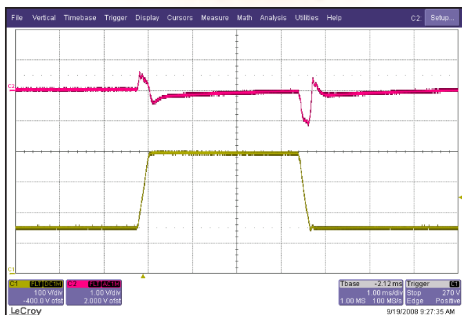
Figure 13: Output voltage response to step-change in input voltage (155 V - 400 V - 155 V) in 250 \mu s. Load cap: 10 \mu F, 100 m \Omega ESR tantalum cap and 1 \mu F ceramic cap. Ch 1: Vin (100V/div). Ch 4: Vout (1V/div).
