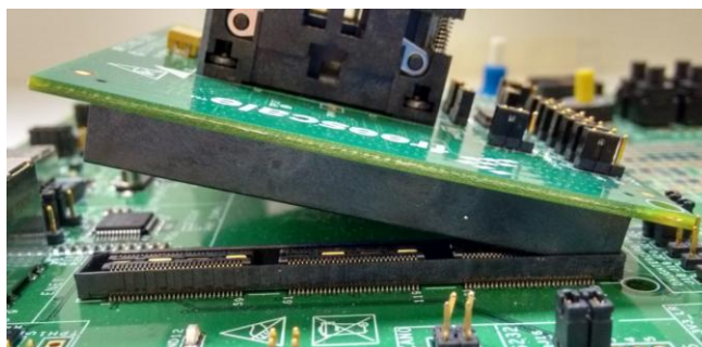
Figure 3. Removing a daughtercard
