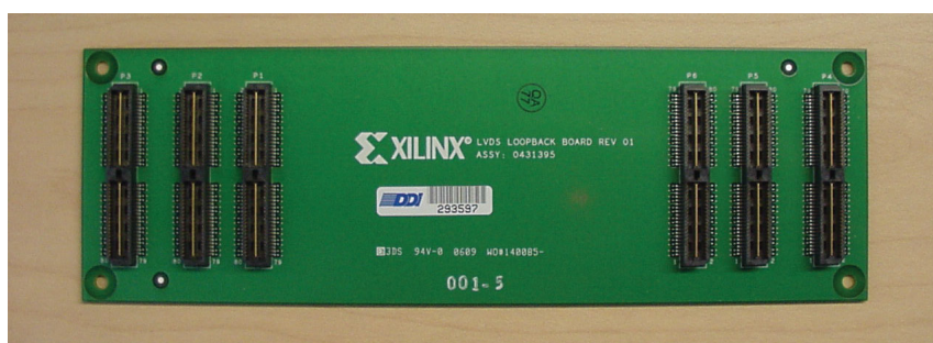
Figure B-1: Xilinx LVDS Loopback Board
