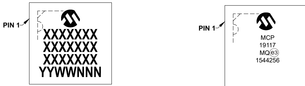
28-Lead QFN (5x5x0.9 mm) ( MCP19117 only )
