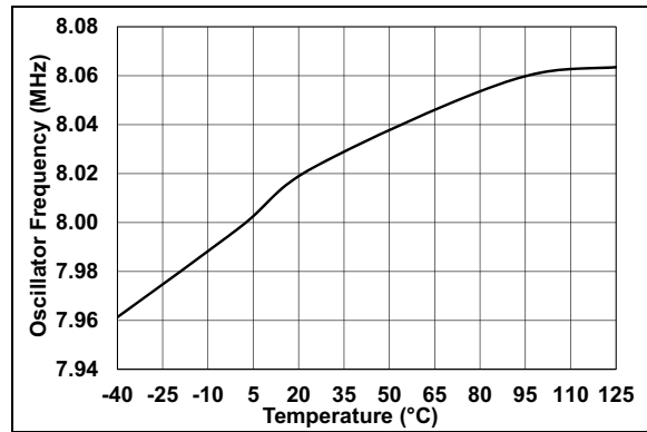
FIGURE 7-12: Oscillator Frequency vs. Temperature.
