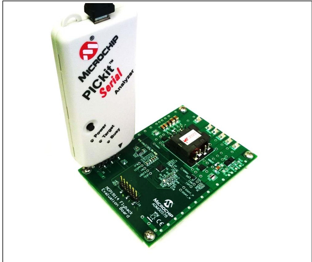
FIGURE 3-1: PICKit Serial Analyzer Connection to the Board.
