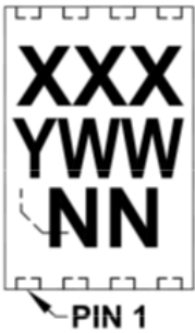
8-Lead DFN (2x3x0.9 mm)
