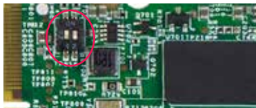
Figure 2. SW602 setting for internal boot mode
