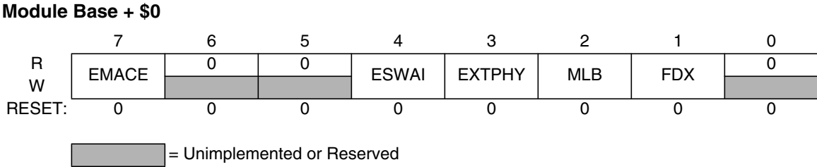
Figure 11-2. Network Control (NETCTL)
