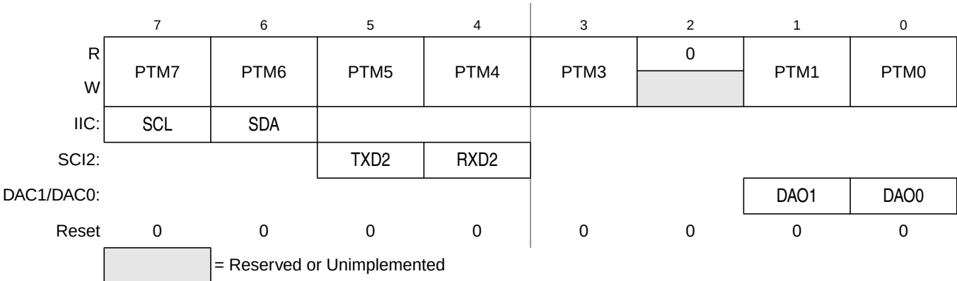
Figure 3-10. Port M I/O Register (PTM)
