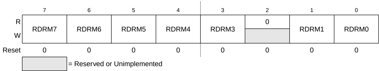
Figure 3-13. Port M Reduced Drive Register (RDRM)
