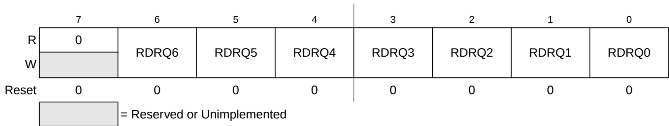
Figure 3-26. Port Q Reduced Drive Register (RDRQ)
