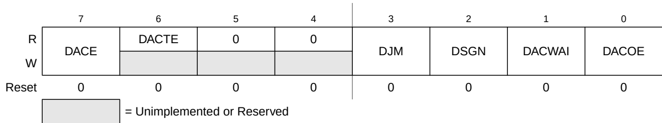
Figure 7-3. DAC Control Register 0 (DACC0)
