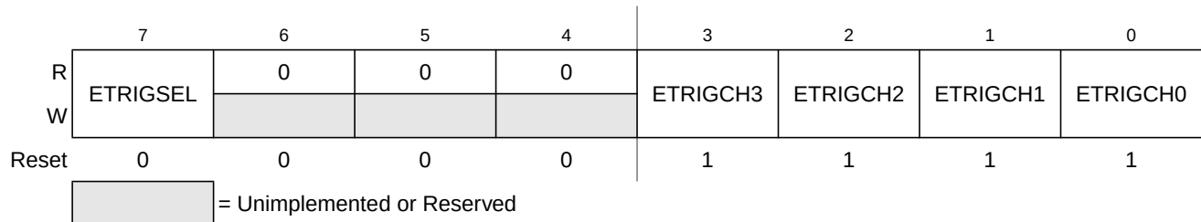
Figure 6-4. ATD Control Register 1 (ATDCTL1)
