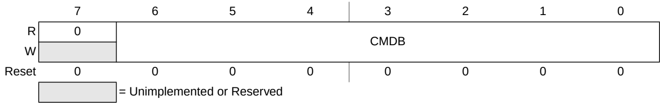
Figure 2-12. Flash Command Register (FCMD - NVM User Mode)
