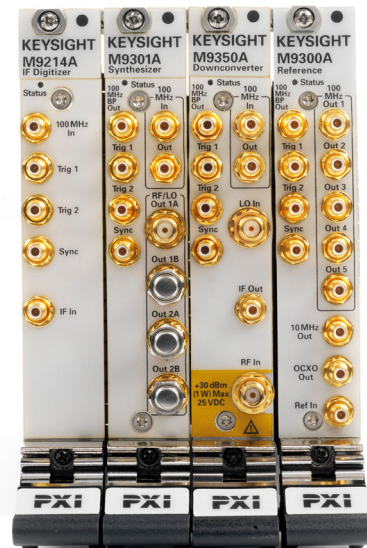
Figure 1. M9391A PXIe vector signal analyzer with four modules consisting of the M9214A digitizer, M9301A synthesizer, M9350A downconverter and M9300A frequency reference.
