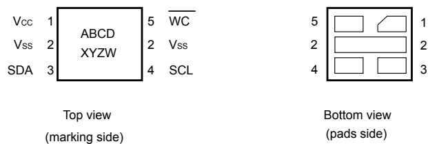
Figure 3. UFDFPN5 (DFN5) package connections
