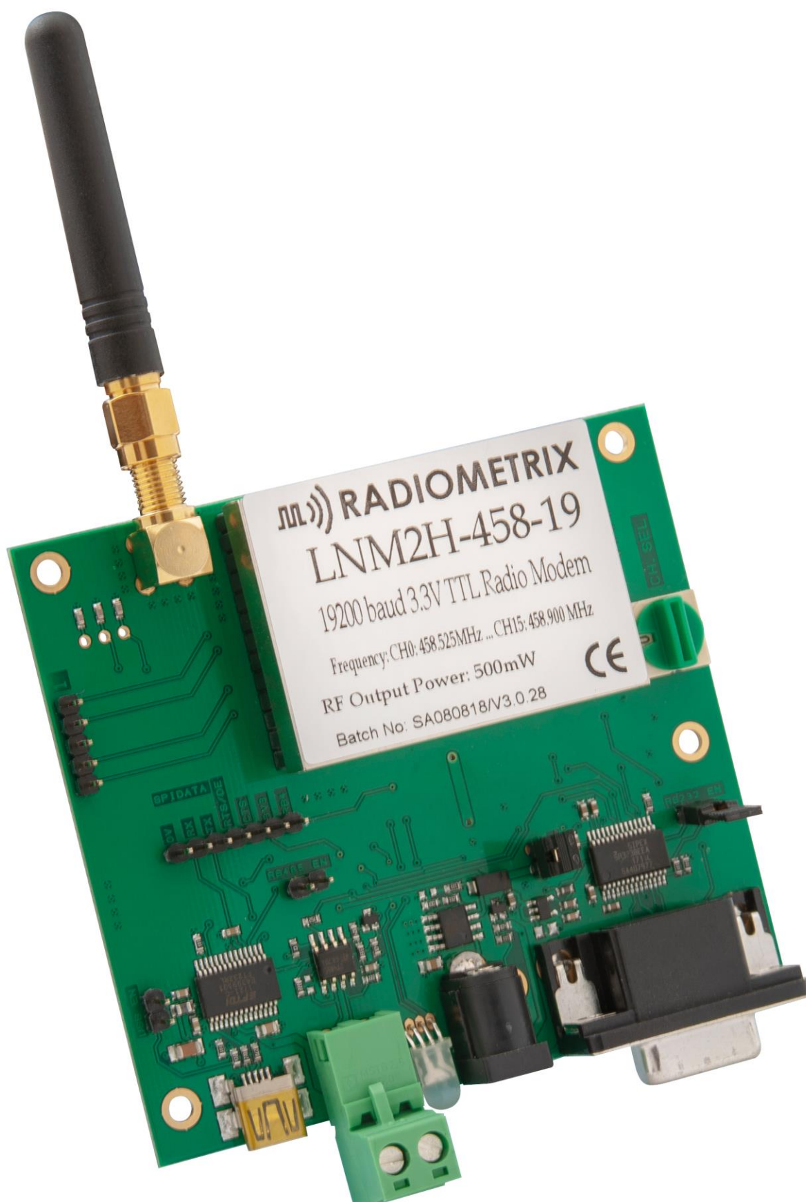
Figure 3: LNM2H/LNM3H Evaluation Kit with RS232, RS485 and USB interface
