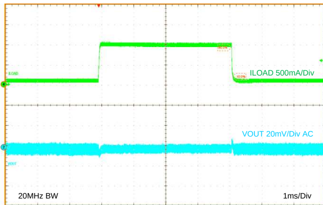
Figure 60. Load Transient V_{OUT} = 3.3\text{ V}
