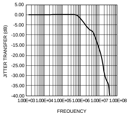
Figure 10. Jitter Transfer Curve
