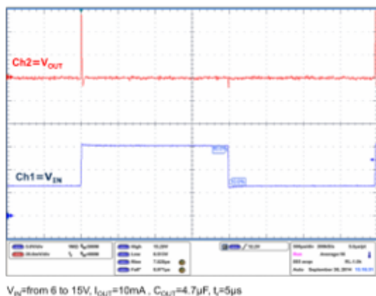
Figure 24. Line transient ( V_{OUT} = 5\text{ V} )
