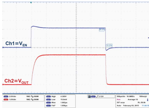
Figure 27. Startup with enable ( V_{OUT} = 3.3\text{ V} )
