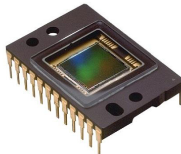
Figure 1. KAI-1010 Interline CCD Image Sensor
