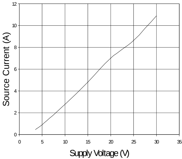
Fig. 22 Output Source Current vs. Supply Voltage
