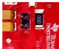
Figure 14. Current Measurement Point
