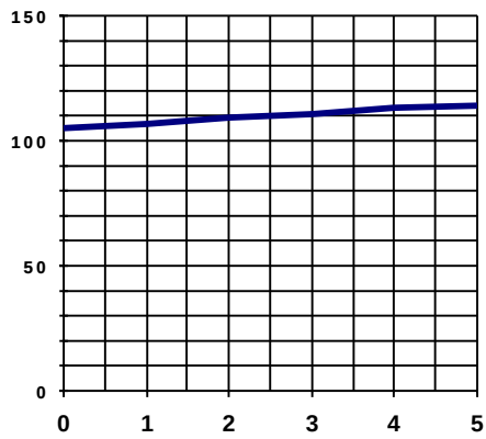
Figure 9 - R ds(on) (mΩ) Vs I out (A)
