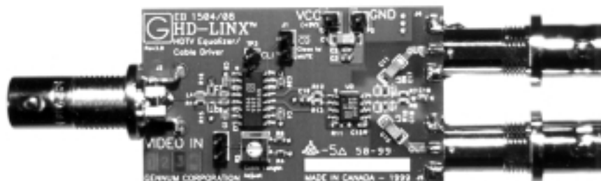
Fig. 34 Photograph of GS1504/GS1508 Evaluation Board
