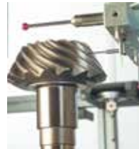
Pinion gear tooth surface measuring
