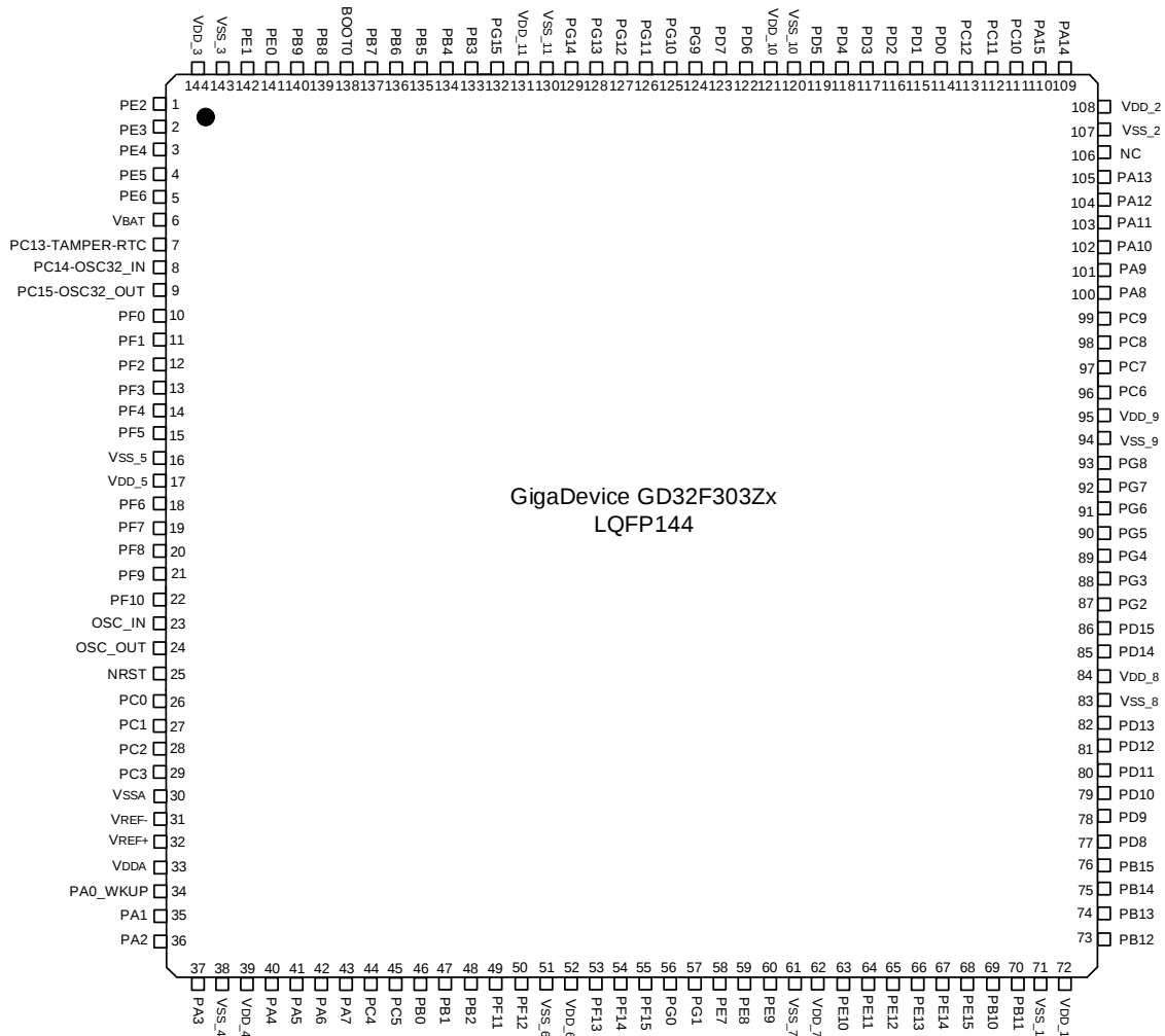
Figure 2. GD32F303Zx LQFP144 pinouts
