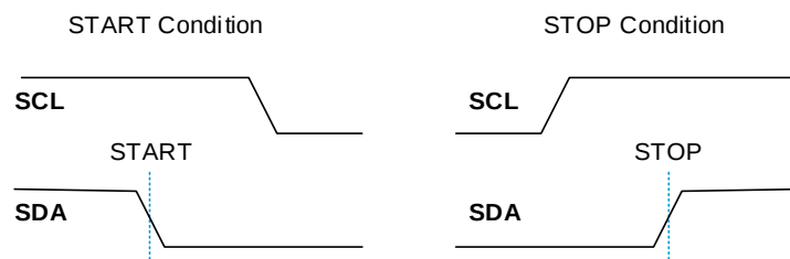
Figure 5. START and STOP Condition Waveform
