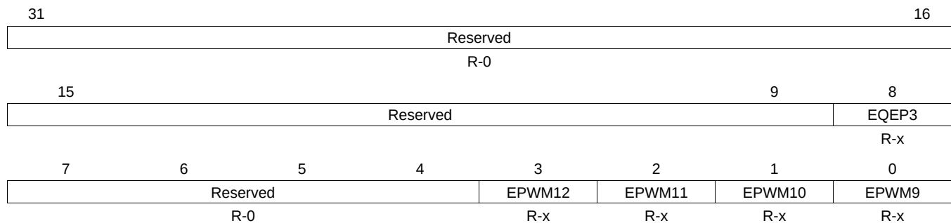
Figure 1-46. Control Subsystem Peripheral Configuration 2 (CCNF2) Register
