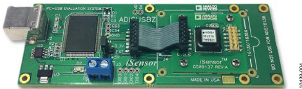
Figure 3. ADIS16265/PCBZ and ADISUSBZ
