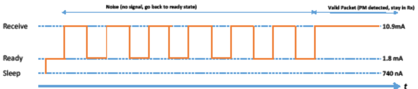
Figure 4.23. Preamble Sense Mode
