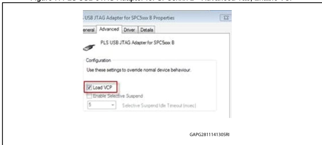
Figure 7: PLS USB JTAG Adapter for SPC5xxx B - Advanced Tab, Enable VCP
