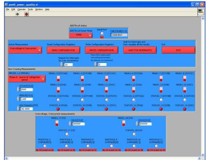
Figure 24. Overvoltage and Overcurrent Measurements Panel
