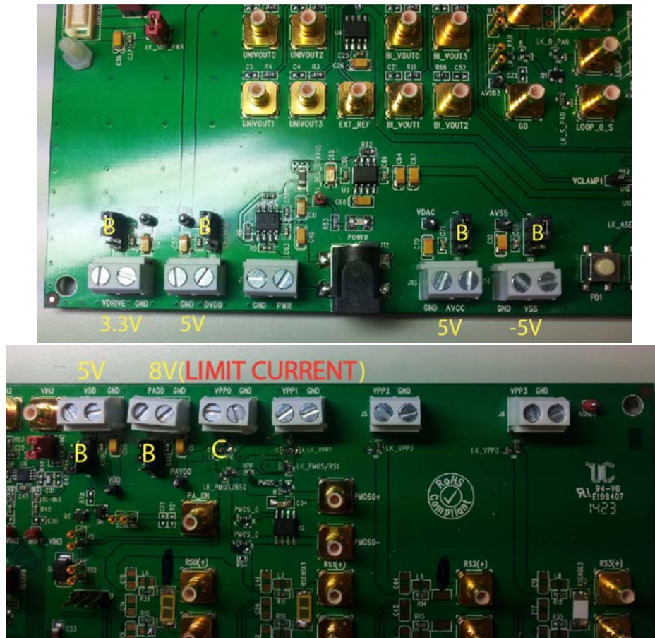
Figure 3. EVAL-AD7293SDZ Power Connections
