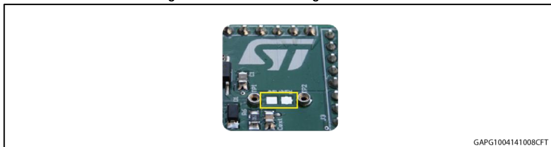
Figure 5: Pads for soldering SMD resistor
