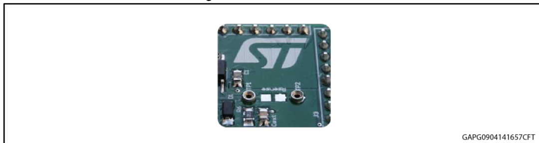
Figure 4: Mounting through-hole sense resistor
