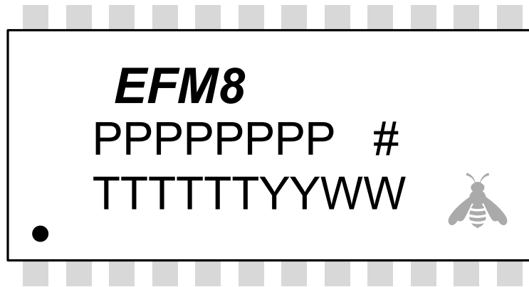
Figure 7.3. QSOP24 Package Marking
