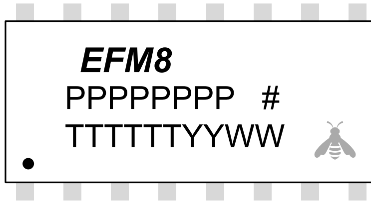
Figure 9.3. SOIC16 Package Marking
