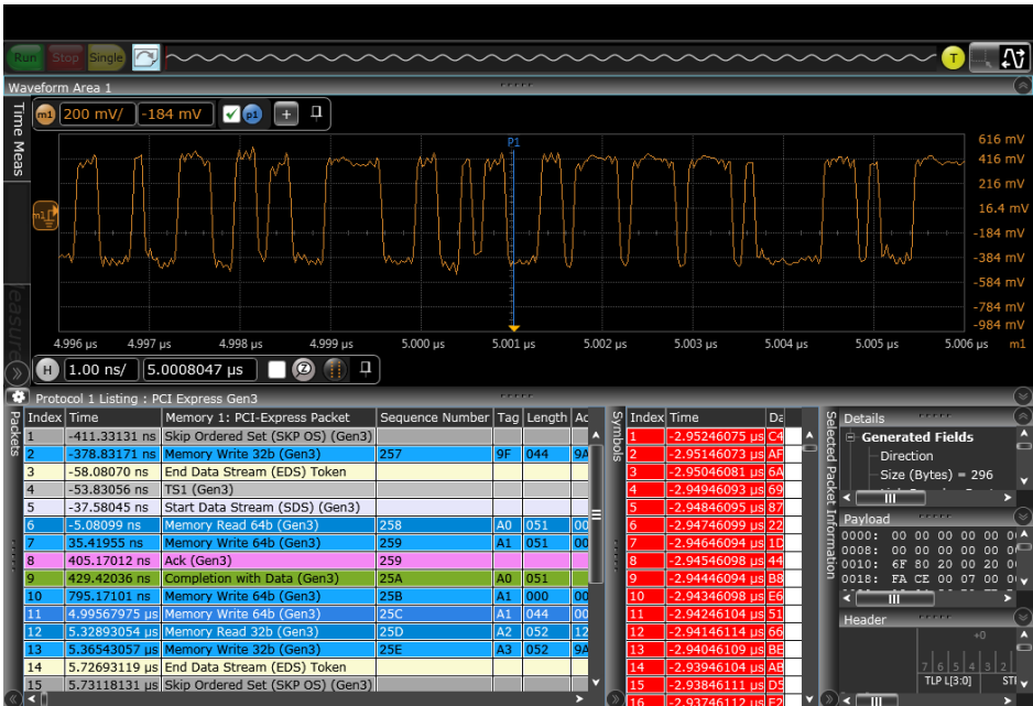
Z-Series decoding the PCI Express Gen 3 packets.
