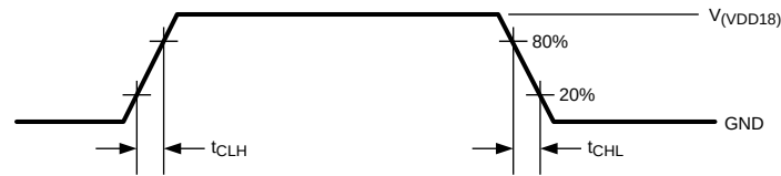
Figure 1. LVCMOS Transition Times
