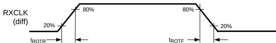
Figure 4. LVDS Output Transition Time
