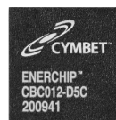
5 mm x 5 mm DFN SMT Package
