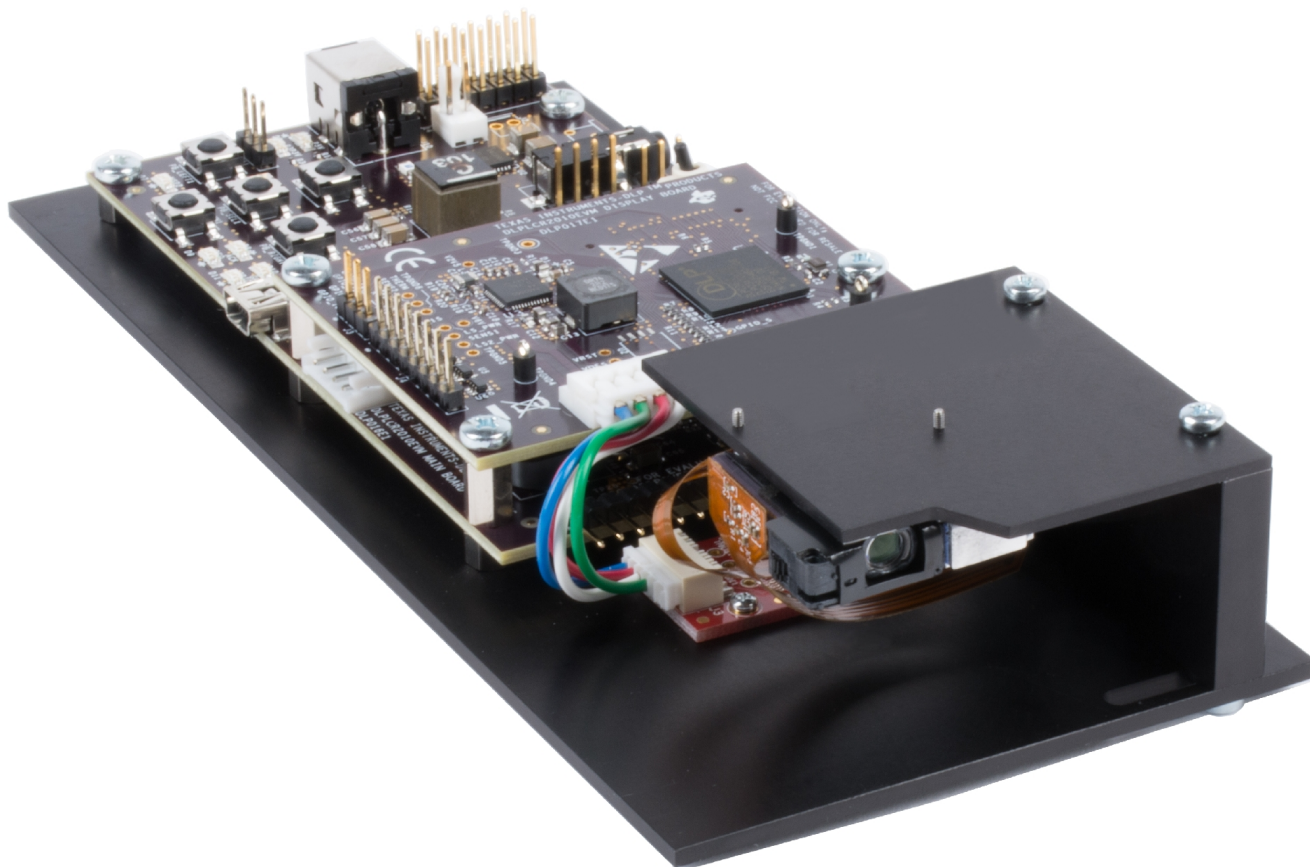
Figure 8. DLP2010 Light Control complete EVM
