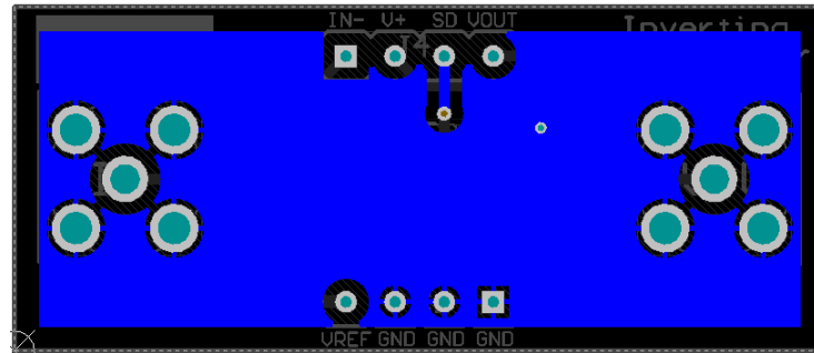
Figure 32. Inverting Comparator Bottom Layer
