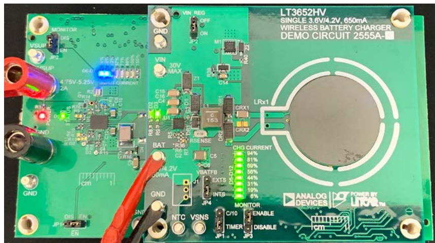
Figure 3. DC2555A-A-KIT in Operation
