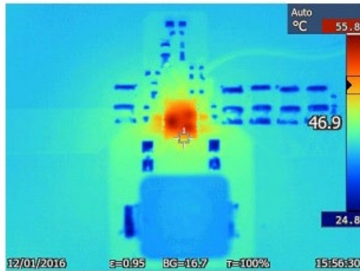
Figure 4. Thermal Image for a 3.6V Input Converter Delivering 5V at 3A
