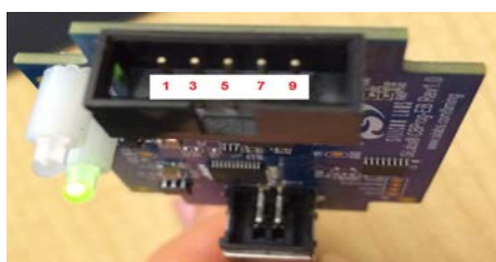
Figure 4.15. Interface Pins on Header (Front View of CBPROG-DONGLE)
