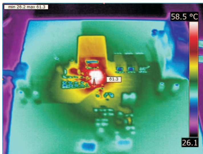
Figure 12. CSD86350Q5DEVM-604 Thermal Image
