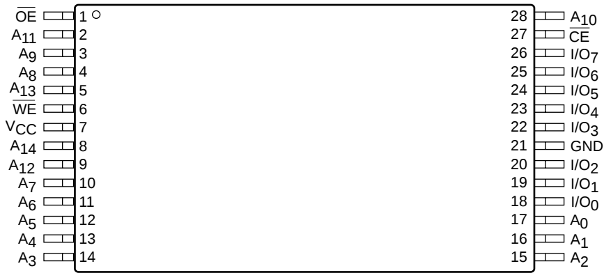
TSOP Top View (8mm X 13.4mm) (H)
