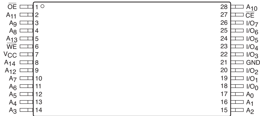
TSOP Package (8mm X 13.4mm) (T13, H13)
