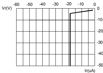
FIG.3b BLUE & GREEN REVERSE CURRENT VS. REVERSE VOLTAGE.
