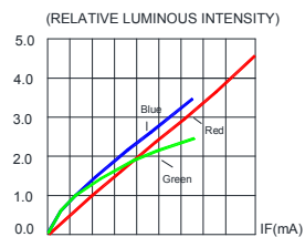
FIG.2 RELATIVE LUMINOUS INTENSITY VS. FORWARD CURRENT
