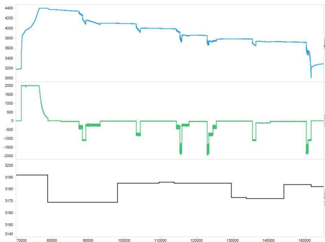
Figure 9-2. Full Charge Capacity Tracking (X-Axis Is Seconds)
