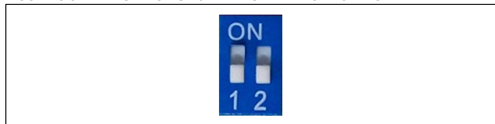
FIGURE 3-37: SWITCH SW9 IN FLASH APPLICATION MODE
