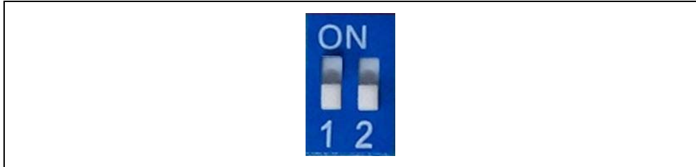
FIGURE 3-1: SW9 IN FLASH APPLICATION MODE
