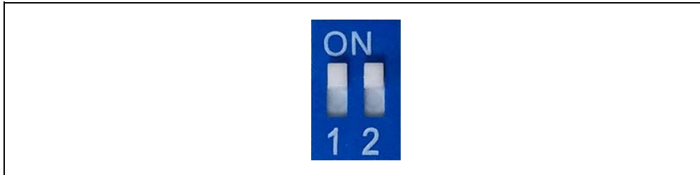
FIGURE 3-38: SWITCH SW9 IN ROM TEST MODE
