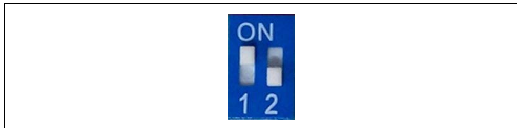
FIGURE 3-31: SWITCH SW9 IN FLASH TEST MODE
